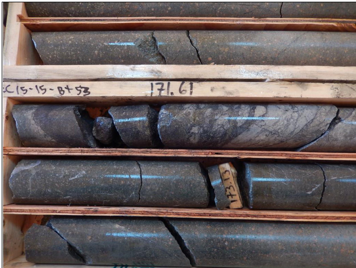
Figure 6-12: P2 Vein and Stockwork Zone Intersection in Hole CC15-15
